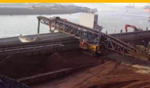
65 METERS OF MOBILE CONVEYOR BELT FOR THE TRANSHIPMENT OF IRON ORE AT CORUS IN IJMUIDEN, CAPACITY OF 3000 TONNES/H
