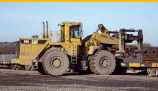
CATERPILLAR 990 USED FOR THE TRANSPORT OF STEEL SLABS AT A STEEL PLANT IN IJMUIDEN
